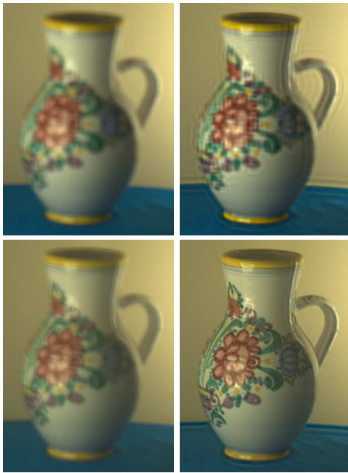
Figure 15: Comparison of traditional focus deblurring with a mask in the aperture. (Top) Captured blurred photo and the deblurred image for open aperture. (Bottom) Captured blurred photo and the deblurred image using the 7 \times 7 mask in the aperture.
