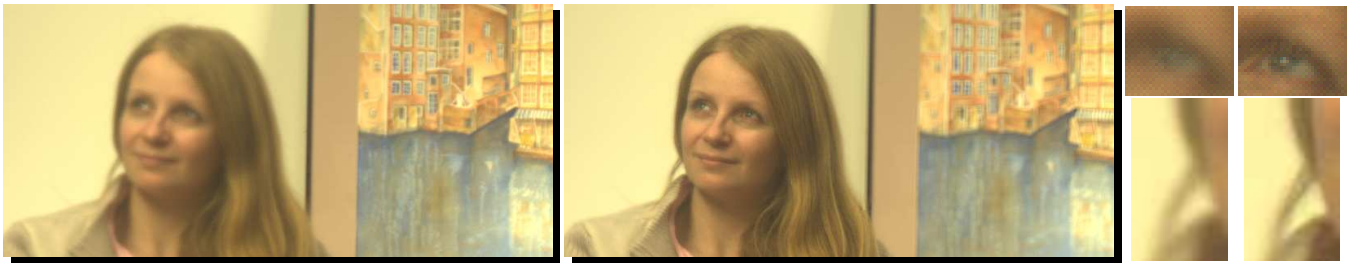
Figure 11: Full resolution digital refocusing using Encoded Blur camera. (Left) Captured image where both the person in front and the painting are blurred. (Middle) Refocused image, the person has been brought into focus. (Right) Since the defocus PSF is made broadband by inserting a broadband mask in the aperture, deconvolution can recover fine features such as the glint in the eye and the hair strands.
