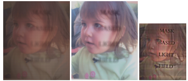
Figure 8: Our light field camera can be used to refocus on complex scene elements such as the semi-transparent glass sheet in front of the picture of the girl. (Left) Raw sensor image. (Middle) Full resolution image of the focused parts of the scene can be obtained as described in Section 3.6. (Right) Low resolution refocused image obtained from the light field. Note that the text on the glass sheet is clear and sharp in the refocused image.
