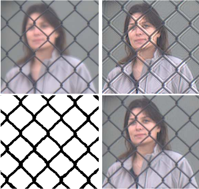
Figure 12: Deblurring in presence of partial occluders. (Top Left) Blurred photo of a person occluded by the in-focus fence. (Top Right) Deblurring without taking the occluders into account results in artifacts. (Bottom Left) Binary mask for the occluders. (Bottom Right) By solving the weighted deconvolution equation, one can remove these artifacts.
